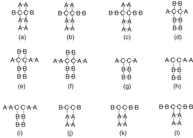
Figure 22. Twelve kinds of diatomic C molecule cluster, where the diatomic C molecules in (a)–(f) are inside systems and those in (g)–(l) are on boundaries.
